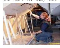
definitely a case of 'Block Planes 'R' Us' as they were definitely the tool of choice. Over left again Sophie is shoring up a dummy plank to test the bevels.
