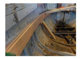
damage in her starboard riser has been cut out with new timbers prepared ready to go back in. Over left the final layer of the Port riser is being sprung into place and below right Jim is applying his fairing skills to the after end in anticipation of Fred coming along to take the glory and do the last two minutes. Talking of whom, who
