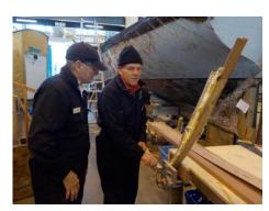
take a well earned rest. He does look comfortable though doesn't he? Change of shift again, above left Whaler John and Graham are back on the job and are cleaning up the laminated frame out of the boat before it is trimmed and fitted with a couple more sacrificial laminates that they can plane down to fit the camber of
