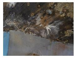
the boat. As a point of interest in the photo over left shows a good example of the spores of the dry rot as they spread across the surface of the timber between the laminates of the 2007 riser and the hull. Scary isn't it, more like the monster from the deep. Just over right Graham A and David S are taking out one of the king posts, and over left David is holding the beast in his arms and it is
