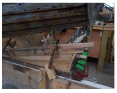
she was only there for one day. In the meantime Tom is catching up on notes left by David and over right the output of all of this effort is the fitting of three planks on the port side and three on the port. As you can see we are using repaired original planking wherever possible by fitting graving pieces in. Over left Brian D and Linden are in discussion on
