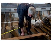
Above left David S is swinging off the end of his hammer and bolster chisel as he cuts away the rotten concrete, whilst in the middle b above he has started to lay down the plywood pattern ready to mark and cut all of the bolt positions. We will use this later to transfer all of the hole positions onto our new keelson ready for drilling. Over right above he is doing his fine tuning before he 'hacks out the holes.
