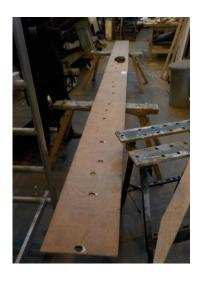
Finally the patterns were located onto the new prepared timber and tacked in place, this just left one final fine tune on the hole positions before the new keelson was drilled. On this section we had six centre line datum viewing holes and ended up with cross hair sightings for each bolt hole. When it is drilled if our calculations are right the new
