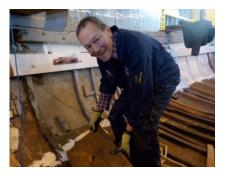
These baulks of timber weren't the only bits that needed removing from the bilges before we could get the keelson completely out, there was also quite a bit of concrete that had been put in over the years to stop the leaks, most of that was taken out as well.
