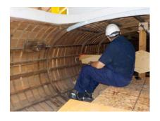
Over left you can see Steve sitting just aft of where the engine would have been located. The engineer had a tiny slatted wooden seat 13inches long x 8 inches wide. He may have got one cheek of his rear end on it if he was lucky. This was fixed to the inside of the hull alongside his engine to sit on when he wasn't tweaking the roaring beast. The Captain was much luckier he had the whole of the torpedo warhead on which to sit as he conned the boat, lucky old tosh wasn't he.
