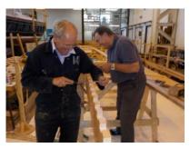
As well as making headway with the engine bearers we also made a start making the laminated stem, this involved machining 30 off 5mm thick veneers out of oak planks and making a very solid moulding jig.
