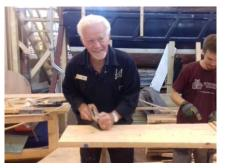
In the photo above left and middle Steve and Jacques are thinning down the joint area ready to mark out and cut the scarf joints. The forward sections are 2inches thick as they take the full weight of the engine and the tails are down to 1 ¼ inch thick as part of the designed weight saving process. I suppose you could say that this is a 'taking off day.
