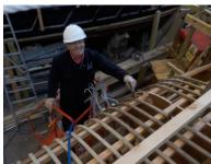
In the photos below some of the other work that has been taking place, below left JohnP and Keith's infills are all in place and they have started to fair off all of the sticky out bits, here they have fitted a temporary fairing batten to check the line, looking along the batten shows that we still have a bit more tweaking to do to get the slight curve out of it.
