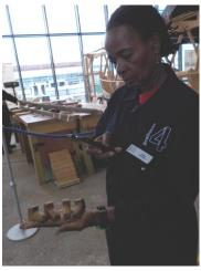
necessary to stop the bottom boards floating away. Above centre Fay is cutting out some toggles for the bottom board closure boards and above right the finished items are ready for a couple of coats of varnish before she fits them into the boat which she is doing over left. Trevor D made up a dozen or so bottom board swivel toggles which clip the bottom boards to the margin boards to hold them in place.
